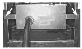
Remove the screws (white arrows) from the tabs on either side of the contactor box.
